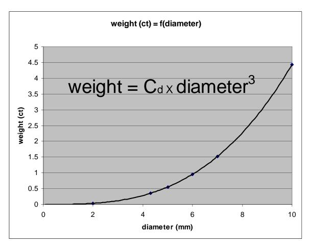
We notice that there is a simple relationship between the diameter and the weight: the weight is directly proportional to the third power of the diameter.
